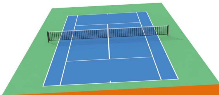
Figure 6. Preferred orientation of slope (side-to-side), if necessary.
